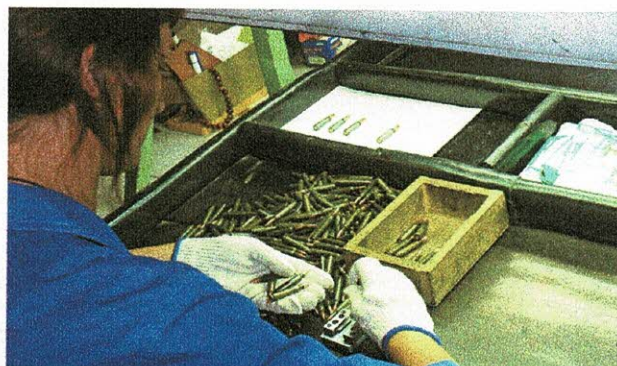
A member of Barnaul's Quality Control team runs a sample of cartridges through a gauge by hand during an inspection to ensure they are within specifications.
