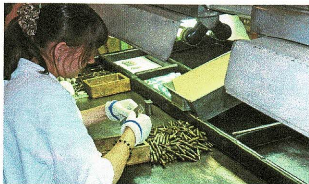
A member of Barnaul's Quality Control team runs a sample of cartridges through a gauge by hand during an inspection to ensure they are within specifications.
