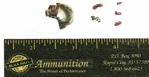
The recovered 7.62x39mm SP had a retained weight of 106.8 grains and had expanded to an average diameter of .656 inch after penetrating to a depth of 16.25 inches.
